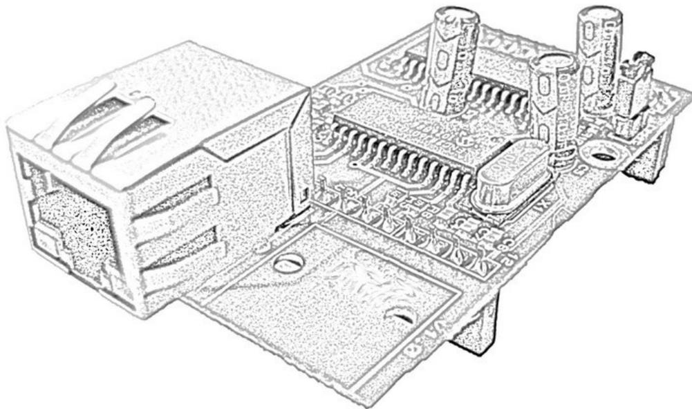
Ethernet to UART / SPI / I2C / IO controller
